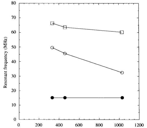
Figure 5: Resonant frequency of the flat-top resonator as a function of position of the movable shorting plate of the additional resonator. The position of the coupling capacitor (Cc) is 11.5 mm. The fundamental frequency is 15 MHz.
