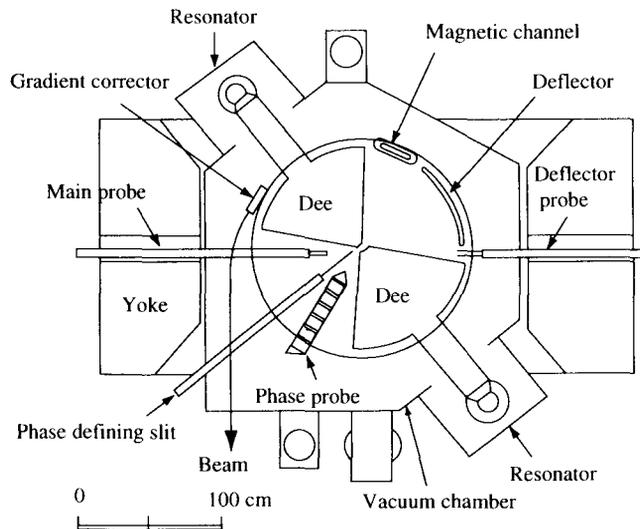
Figure 1: Layout of the AVF cyclotron.
