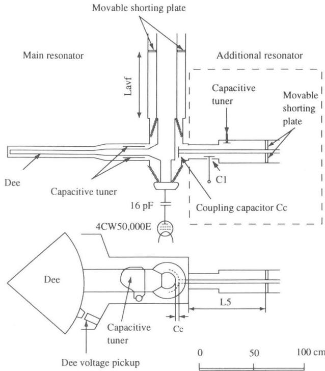
Figure 2: Cross-sectional view of the resonator for the flat-top acceleration system.
