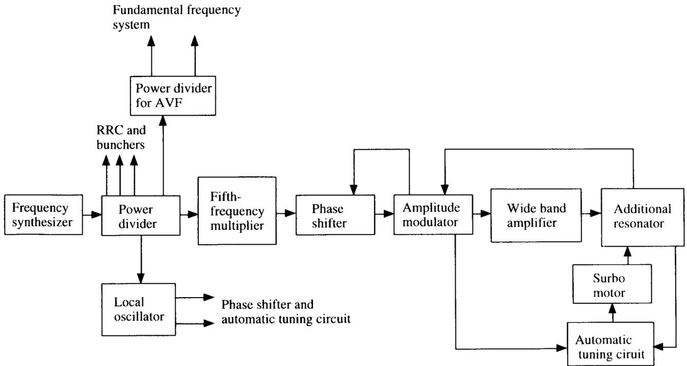
Figure 7: Block diagram of the rf control system for the fifth-harmonic frequency.
