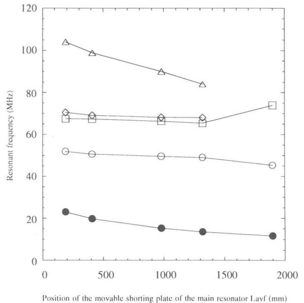
Figure 4: Resonant frequency of the flat-top resonator as a function of position of the movable shorting plate of the main resonator. Closed circles represent the fundamental resonant frequency.
