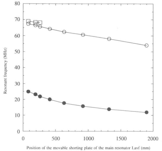
Figure 3: Resonant frequency of the main resonator as a function of position of the movable shorting plate of the main resonator. Closed circles represent the fundamental resonant frequency.
