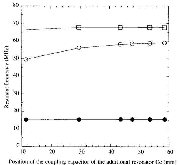
Figure 6: Resonant frequency of the flat-top resonator as a function of position of the coupling capacitor of the additional resonator. The position of the movable shorting plate (L5) is 332 mm.
