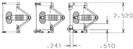
Figure 2: Left to right, cross sections of Mark III, IV and V deflectors. Sparking plates are Stainless Steel for Mark III and Copper for Mark IV and V. Note the water lines in the bases of Mark IV and Mark V. Dimensions are in inches.
