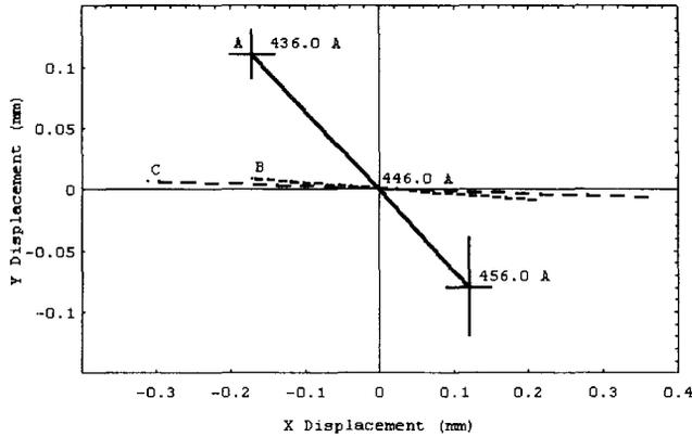
Figure 8: Beam displacement at the inflector exit as a function of the cyclotron excitation current. (A) is measured data, (B) is CASINO data using electric field file INF\_RELAX\_14.DAT and magnet field file MAP29\_DIGI.ZFLD, and (C) is CASINO data using an analytic electric field and magnetic field file MAP29\_DIGI.ZFLD.
