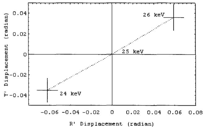
Figure 7: Changes in the angular displacement of the beam at the inflector exit as a function of the injected beam energy.
