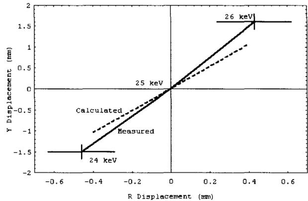
Figure 6: Changes in the Y displacement of the beam at the inflector exit (corresponds to changes in electric bend radius  $A$ ) and the magnetic ( $R$ ) radii of curvature of the injected beam as a function of the injected beam energy.
