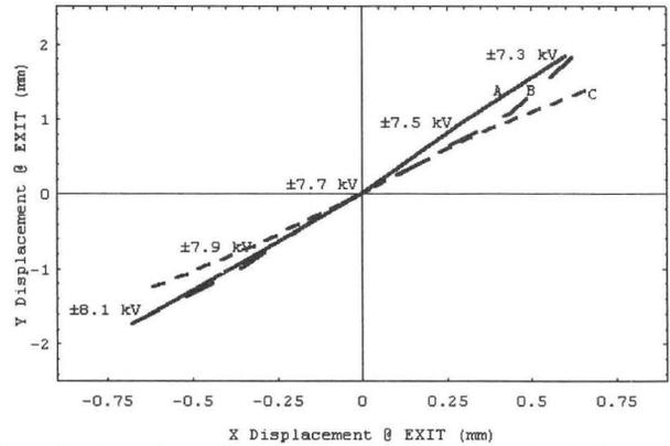
Figure 2: Central ray displacement at the inflector exit scintillator as a function of inflector electrode potential. (A) is measured data, (B) is CASINO data using electric field file INF\_RELAX\_14.DAT and magnet field file MAP29\_DIGI.ZFLD, and (C) is CASINO data using an analytic electric field and magnetic field file MAP29\_DIGI.ZFLD.
