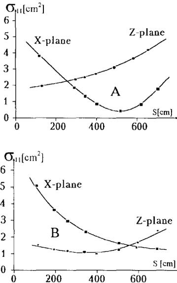
Fig.2 Beam envelope under two modes of the lense operation.
