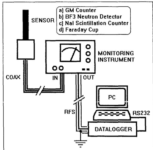
Figure 1: Showing the principle of health physics data acquisition system. The application specific sensors (inset) are connected to the individual monitoring instrument using a coaxial cable (COAX). The analog signal output from the monitoring instrument is linked to the datalogger (in 0-40 mA current loop mode) via a RF-shielded twisted pair cable (RFS). The datalogger is interfaced to the serial port (RS232) of a Personal Computer (PC).
