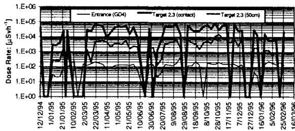
Figure 4: Shows the gamma dose rates at contact (point x in Figure 2) and at 50 cm from the Target Station T2.3 (point y in Figure 2) as well as at the entrance point of the Target vault recorded during the weekly routine Health Physics Survey over the period of 12 December 1994 - 25 February 1996.
