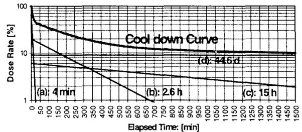
**Figure 3:** The gamma dose rate in the target vault as a function of elapsed time detected with the gamma area monitor GD4 (Figure 2) is shown. The gamma dose detection began immediately after the removal of the proton irradiated copper target plate from the target vault. The initial value of the dose rate ( $t = 0$ ) was normalised to 100%.
