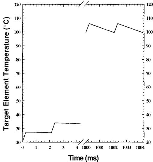
Figure 2: Temperature variation as a function of time experienced by a representative target element in the beam path.
