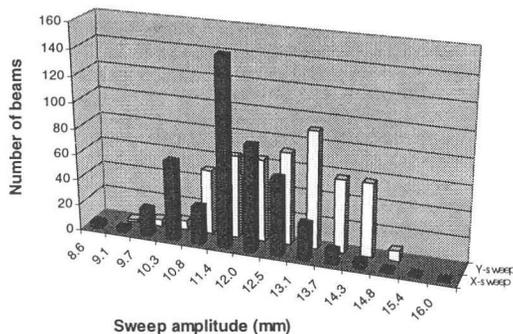
Figure 8: Distribution of sweep amplitudes in the X and Y directions achieved over the period of one year.
