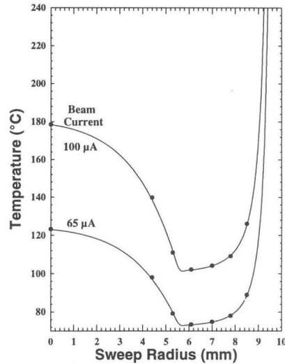
Figure 7: Peak surface temperature in a Zn-target as a function of sweep radius.
