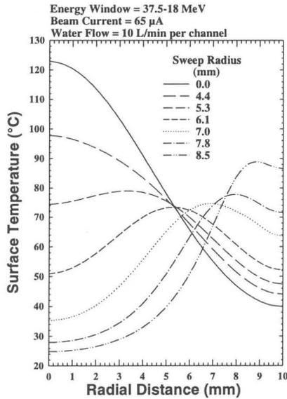
Figure 6: Temperature distributions in a Zn-target.
