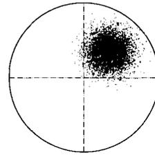
Figure 3: Density plot of a displaced Gaussian beam.
