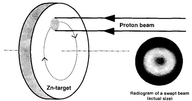
Figure 1: An illustration of how the beam is swept. A radiogram of a foil activated by an 80  $\mu\text{A}$  swept beam is also shown.
