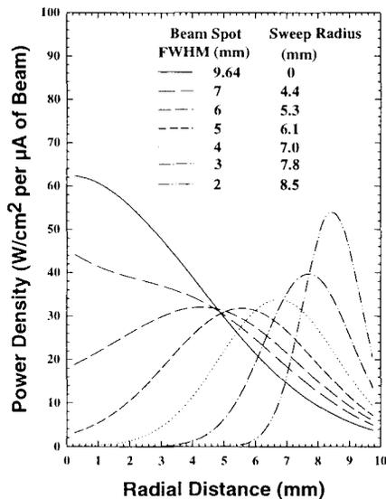
Figure 4: Beam profiles.
