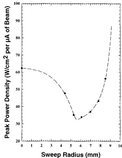
Figure 5: Peak power density as a function of sweep radius.
