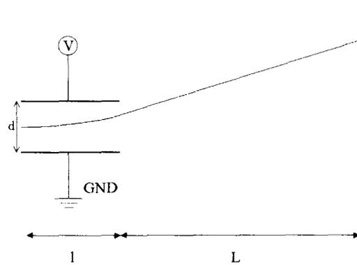
Figure 3: The layout of a beam chopping system.
