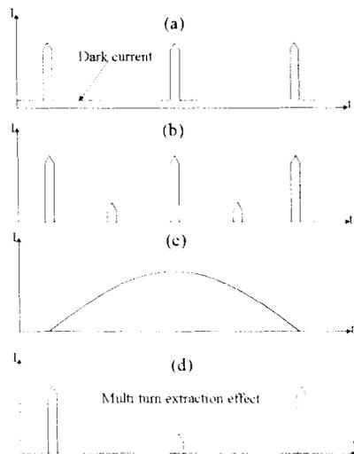
Figure 2: (a) Pulsed beam delivered by the buncher and the rebuncher; (b) Pulsed beam after the Cyclotron; (c) Waveform of the voltage applied to the L.E. Chopper; (d) Pulsed beam with Chopper on.
