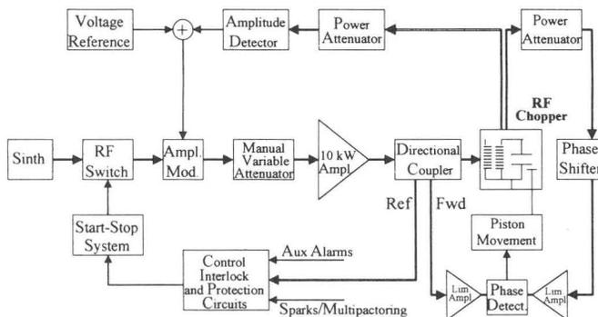
Figure 7: Block diagram of the H.E. Chopper.
