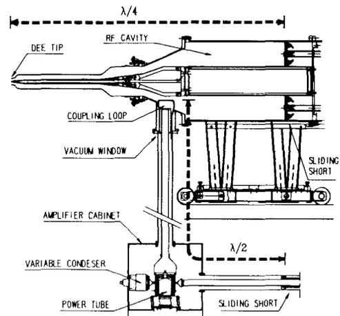
Fig. 1. Schematic cross section of the VINCY Cyclotron RF system with “detuned primary coupling”.
