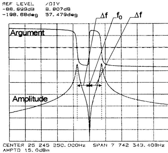
Fig. 2. Frequency response of a resonant coupling RF system (measured at the anode of the power tube) with both resonators tuned to the same frequency.
