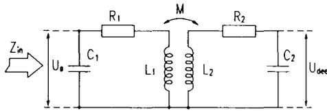
Fig. 4. Lumped circuit approximation of a coupled system.
