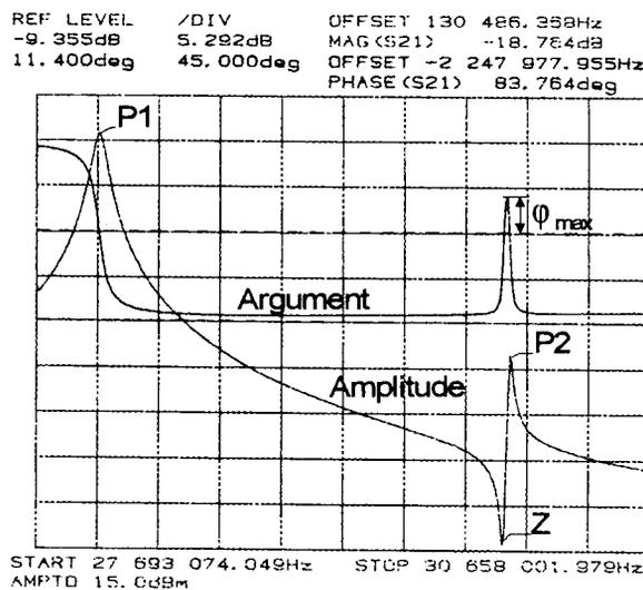
Fig. 3. Frequency response of a system with strongly detuned primary - a working configuration.
