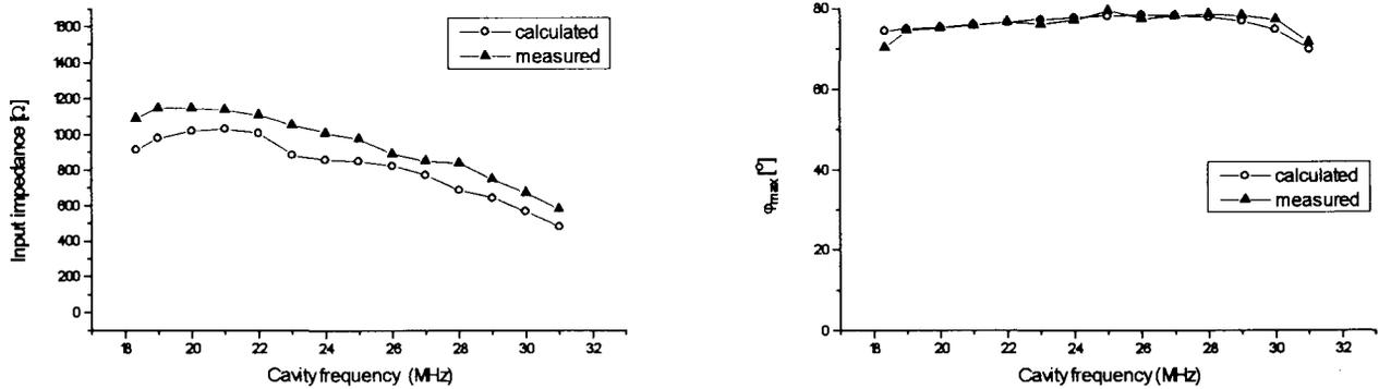
Fig 6. Coupling parameters vs. secondary eigenfrequency for nominal value of the dee-to-anode voltage ratio  $\tau = 20$  dB
