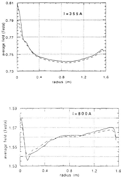
Figure 5 : Average magnetique field Tosca (dotted line) and measurement
