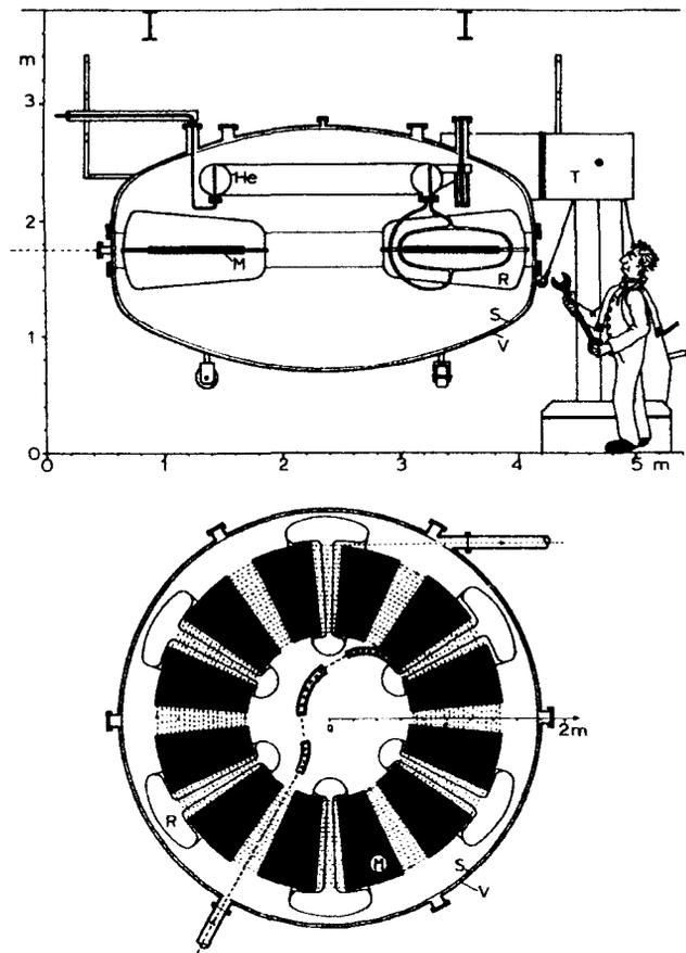
Figure 1. Cross sections of the TRITRON cryostat. V: vacuum vessel, S: 80 K-shield, M: magnet sector, R: rf-cavity, He: helium reservoir, T: support
