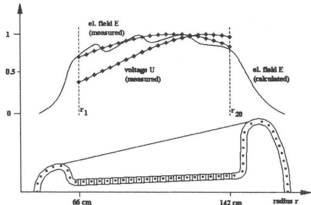
Figure 3. The radial characteristics of the electrical field E (measured and calculated) and voltage U of the cavities.
