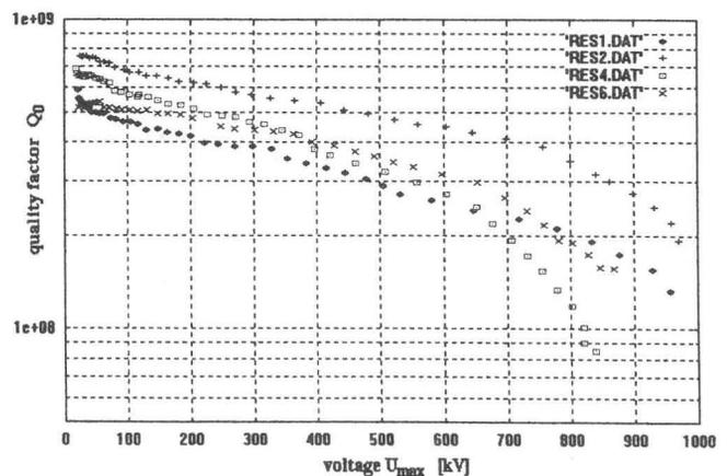
Figure 4. Typical curves of the unloaded quality factor of Tritron cavities versus the voltage amplitude at the last beam hole.
