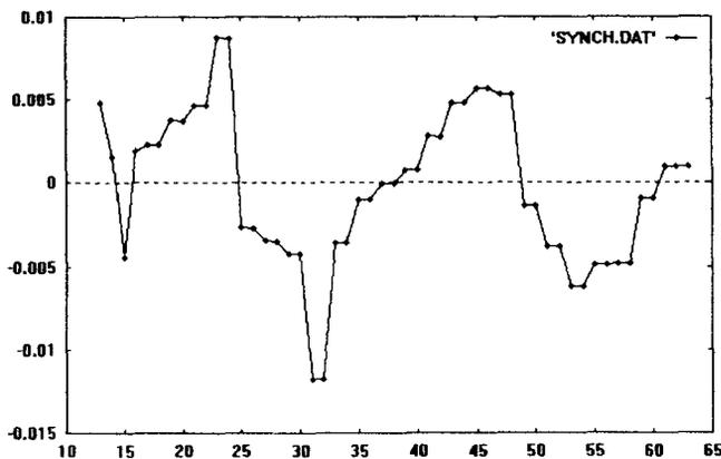
Figure 6. The relative deviations from linear increase,  $\Delta Br/(Br)$ , versus the magnet number of turn 2 to 5, showing two coherent synchrotron oscillations.
