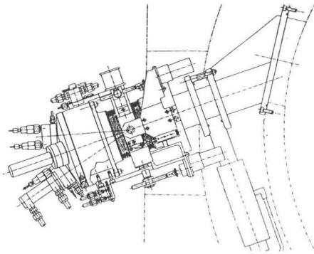
Fig.5 Target Changing Mechanism
