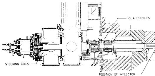
Fig.3 Ion Source and Injection System
