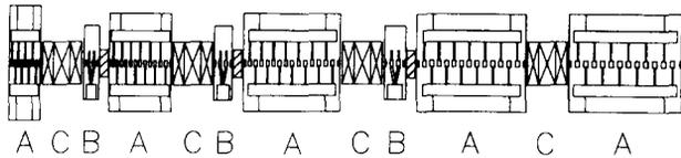
Figure 3: Schematic drawing of the ISAC variable energy DTL. Five IH tanks (A) provide acceleration at  $0^\circ$  synchronous phase, three triple gap spiral resonators (B) provide longitudinal focus ( $\phi_s \sim -60^\circ$ ) and quadrupole triplets (C) provide transverse focus.
