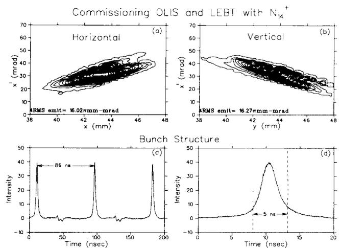
Figure 2: Commissioning results from OLIS/LEBT; the horizontal and vertical emittance of the  $N_{14}^+$  beam and the bunch structure at the end of LEBT.
