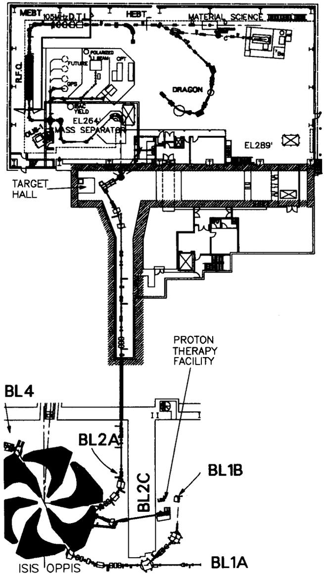
Figure 1: Cyclotron and ISAC Layout.
