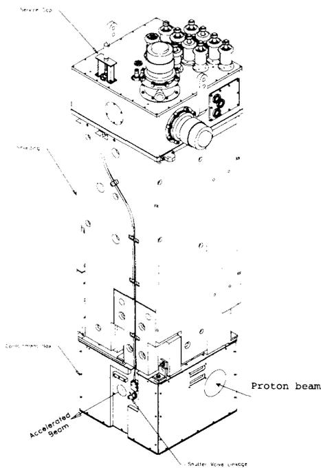
Fig. 4- Three dimensional view of the target module showing the different aspect of the shielding plug concept.
