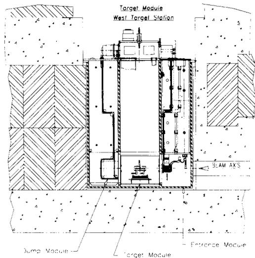
Fig. 2 – Section view of the target station along the primary beam axis.
