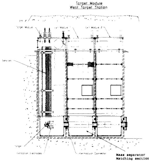
Fig. 3 – Section view of the target station along the heavy ion beam axis.
