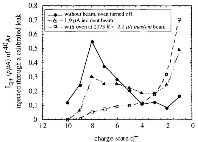
Figure 7 : Charge state distributions of  $^{40}\text{Ar}$  injected through the calibrated leak, obtained with SHyPIE and the two different target systems.
