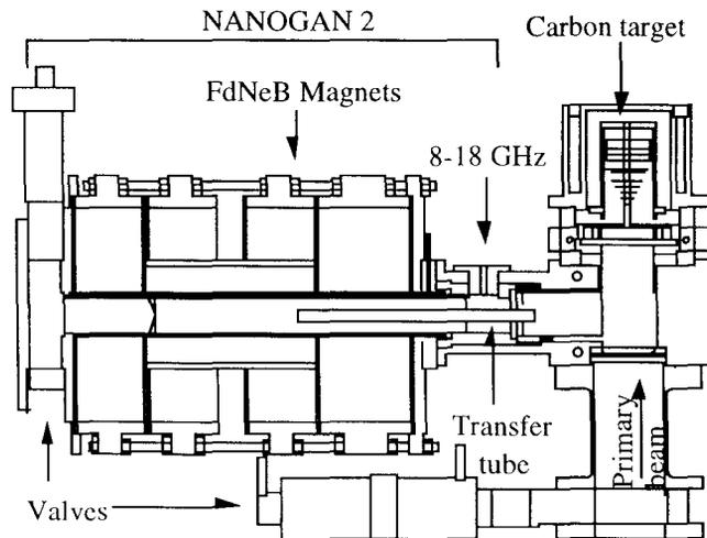
Figure 3: Schematic drawing of the first target ion source system for the spiral project.
