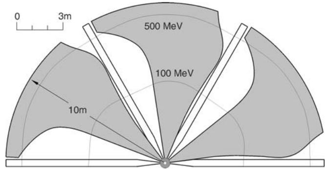
Figure 4: Three sectors of an  $H^-$  separated-sector cyclotron.
