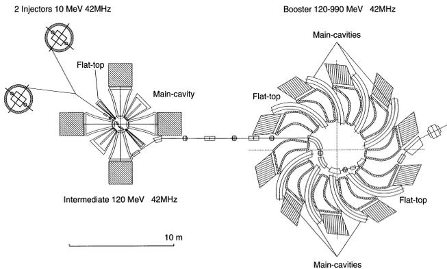
Figure 1: The Energy Amplifier cyclotron complex.
