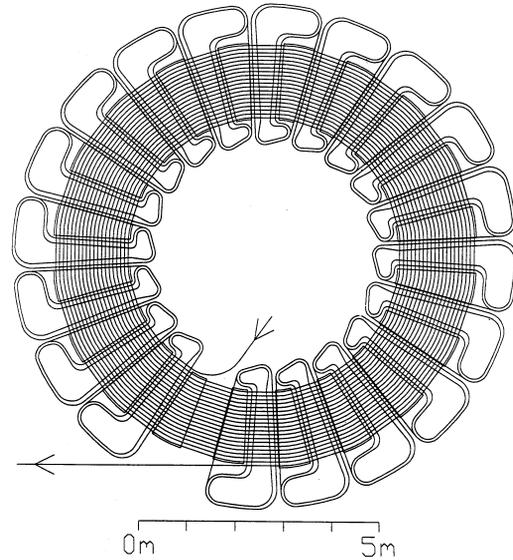
Figure 3: A large separated-orbit cyclotron.
