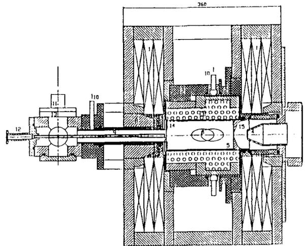
Fig.1 10GHz ECR2 ion source for HIRFL.
