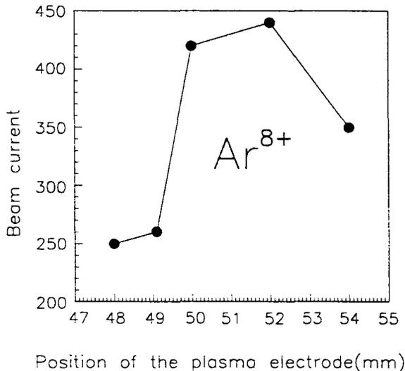
Fig.2 Dependence of  $Ar^{8+}$  beam current( $\mu A$ ) on the position of the plasma electrode.
