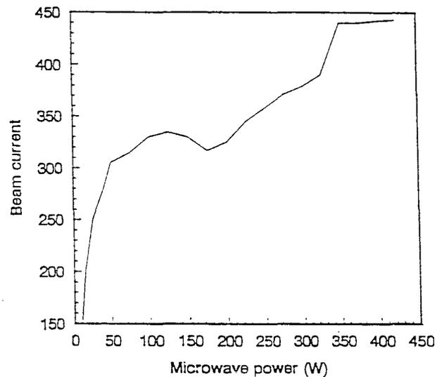
Fig.3 Dependence of  $Ar^{8+}$  beam current( $\mu A$ ) on microwave power.
