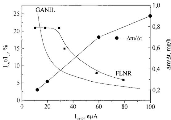
Fig.5 Experimental results for the bunching effect and consumption of metallic  $^{48}\text{Ca}$  versus the ion beam intensity from the ion source.
