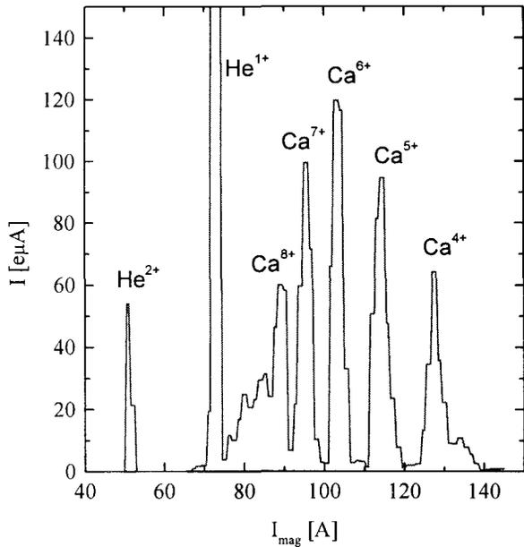
Fig.3 The spectrum of  $^{48}\text{Ca}$  ions optimised for production of  $^{48}\text{Ca}^{6+}$ .
