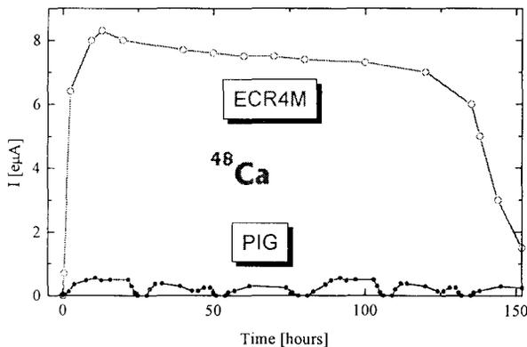
Fig.7 Intensity of the accelerated <sup>48</sup>Ca ion beams from the PIG [13] and ECR ion sources at a physical target.
