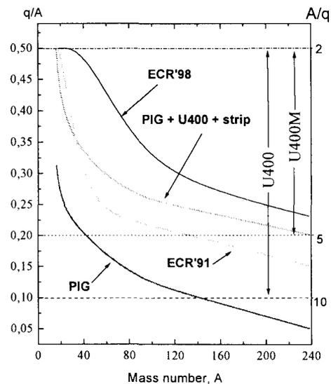
Fig.1 Potentialities of different high charge state and intensive ion sources for cyclotrons.
