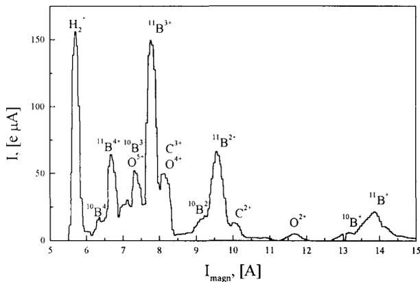
Fig.4 The spectrum of  $^{11}\text{B}$  ions produced from the  $\text{C}_2\text{B}_{10}\text{H}_{12}$  compound.
