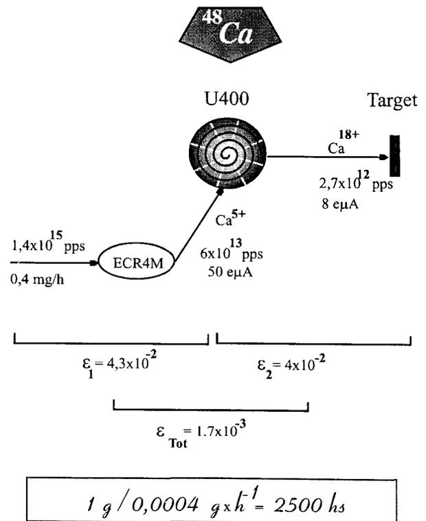
Fig.6. Efficiency of the ECR4M ion source and the U400 cyclotron with the  $^{48}\text{Ca}$  ion beam.
