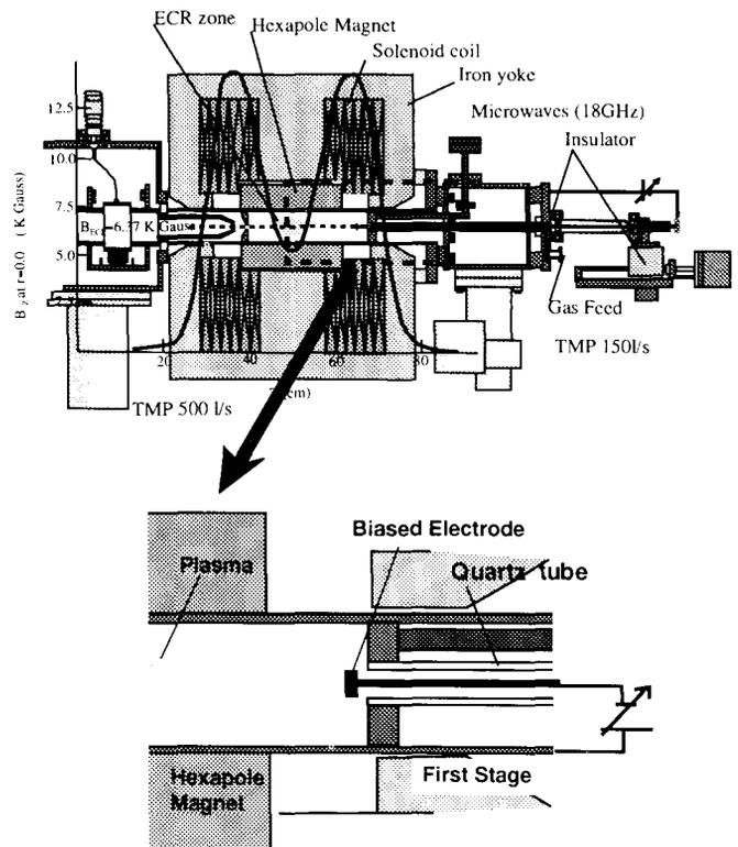
Fig.1 Schematic Drawing of 18 GHz ECRIS with electrode
