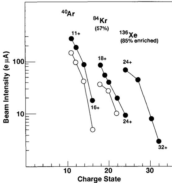
Fig. 6 Beam intensity of highly charged ions from gaseous elements. Open and closed circles are the results without and with using the disc.
