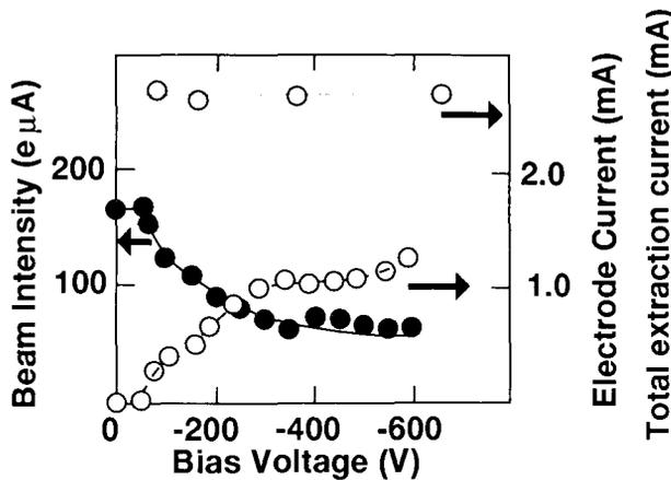
Fig.3 Beam intensity of  $Ar^{11+}$  (closed circles), current of electrode (open circles), and total extraction current as a function of bias voltage
