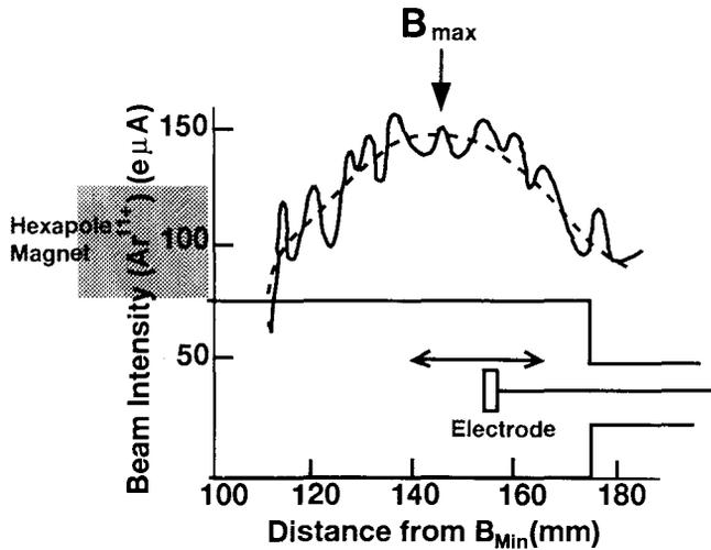
Fig.2 Beam intensity of  $Ar^{11+}$  as a function of electrode position
