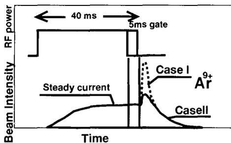
Fig. 9 Beam intensity of Ar<sup>9+</sup> as a function of time under the pulsed mode operation
