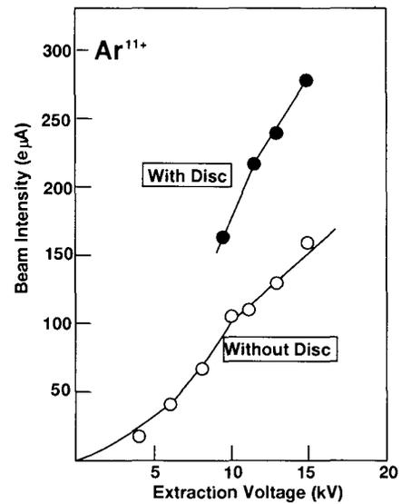
Fig. 4 Beam intensity of  $Ar^{11+}$  as a function of extraction voltage
