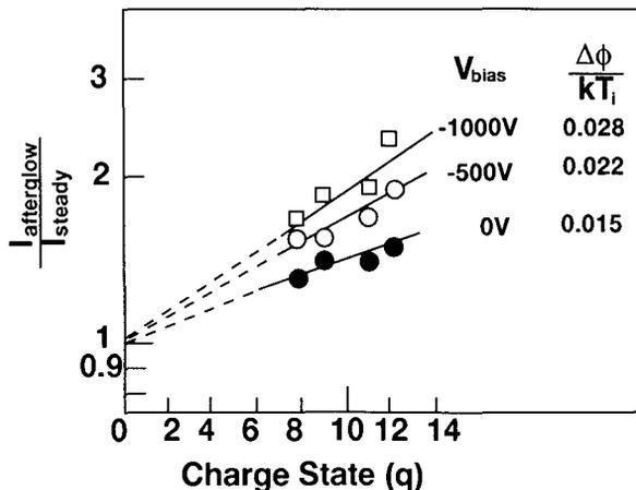
Fig.7 Ratio of afterglow current to steady current as a function of charge state.
