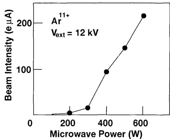
Fig.5 Beam intensity of  $Ar^{11+}$  as a function of microwave power.
