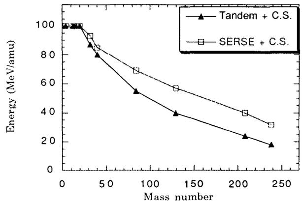
Fig. 3 - The maximum beam energy of the Superconducting Cyclotron.
