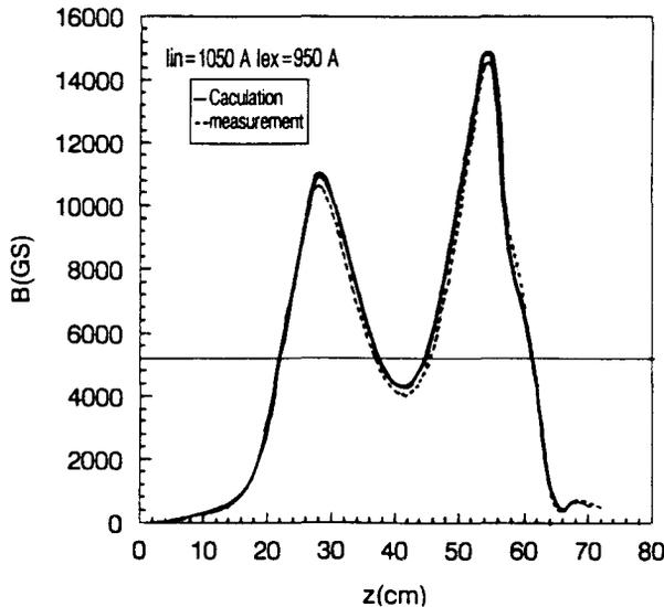
Figure 2 : The axial magnetic field distribution on the axis.
