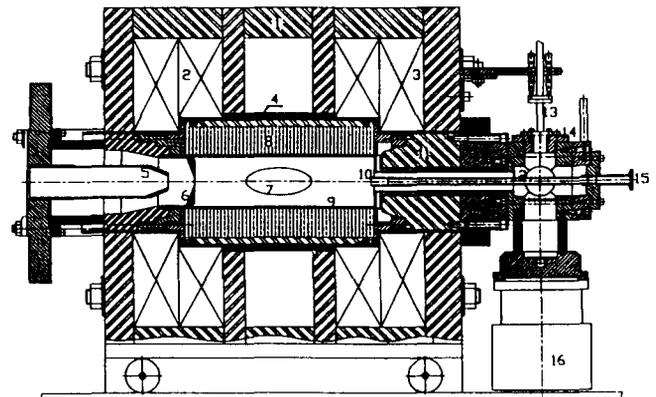
1. Ion yoke 2. Extraction solenoid. 3. Injection solenoid 4. Insulator
