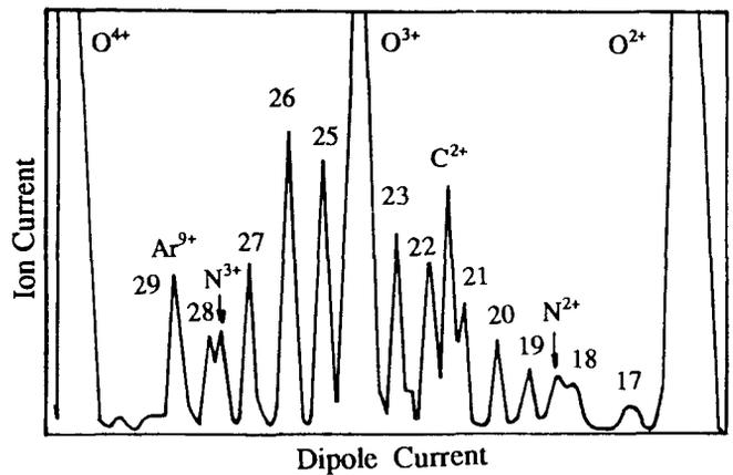
Figure 4 : Xenon-129 spectrum to optimize  $Xe^{26+}$ .
