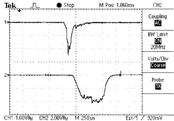
Fig. 4. Upper waveform is ion current for  $\text{Ar}^{13+}$  with ion energy 300 eV per charge of ion, lower waveform is ion current for  $\text{Ar}^{11+}$  with ion energy 100 eV per charge of ion.
