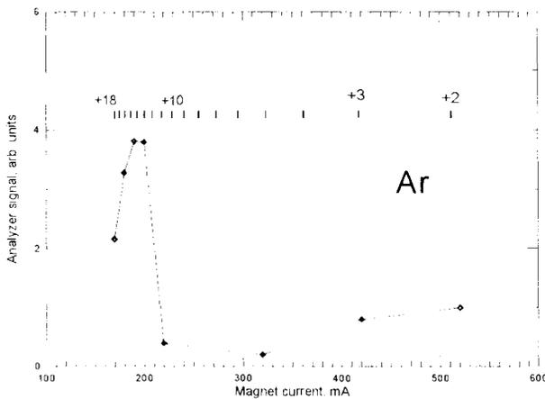
Fig. 5. Dependence of ion analyzer signal on current of analyzer magnet. The magnet currents corresponding the Argon ions with different charges are shown on top.
