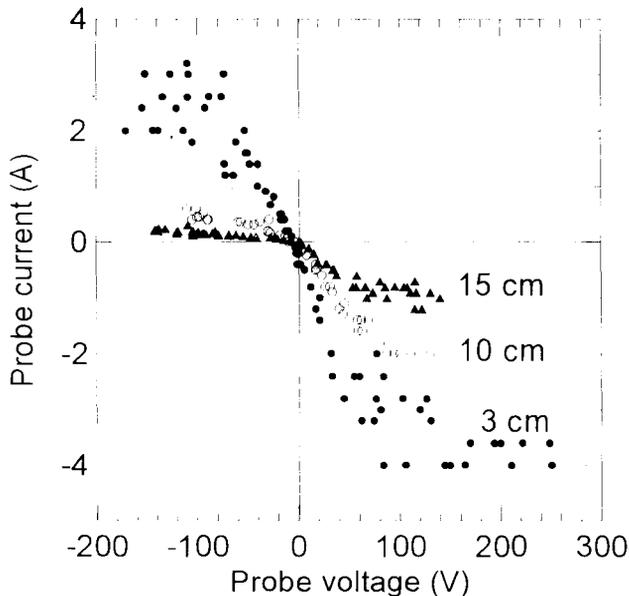
Fig. 6. The volt-ampere characteristics of the probe for different distance between plug and probe.
