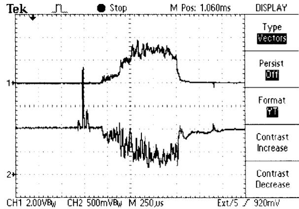
Fig. 3. Upper waveform is the probe current. Lower waveform is transmission factor of diagnostic microwaves through the plasma. sign «2» shows zero level of transmission.
