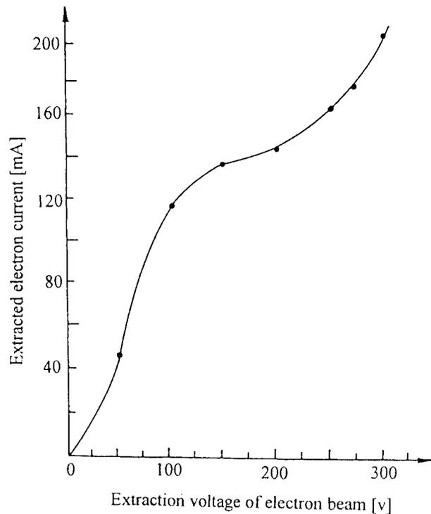
Fig 3. The extracted electron current as a function of extraction voltage.
