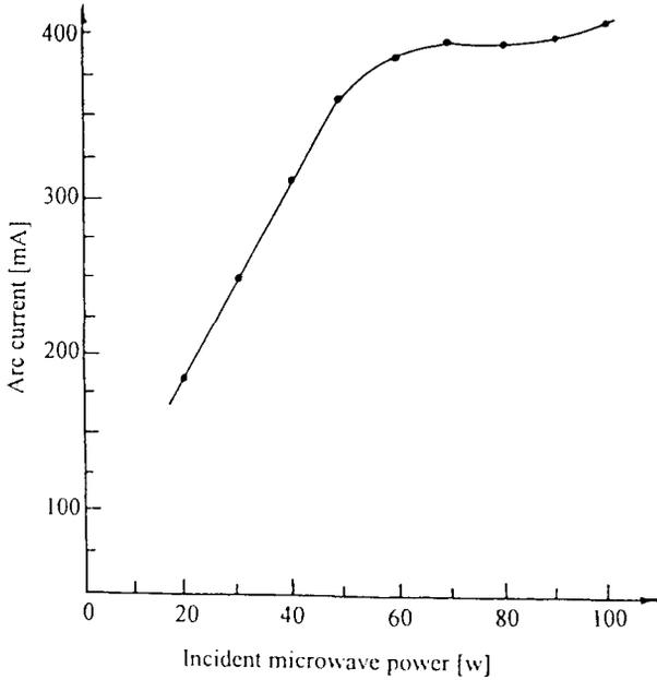
**Fig 4.** The arc current as a function of incident microwave power.
