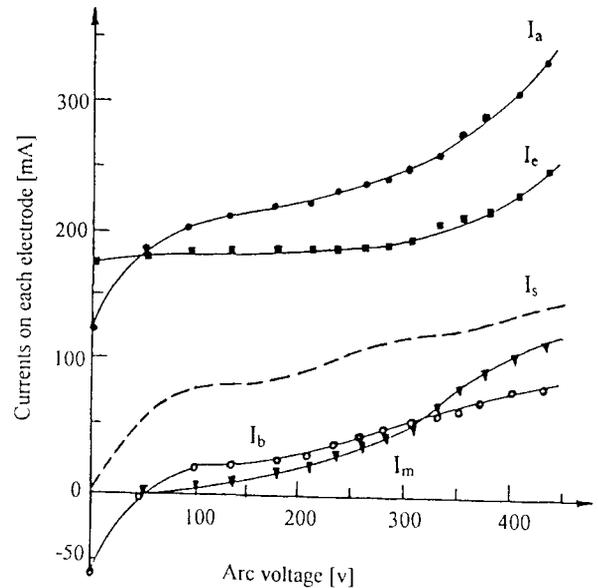
**Fig 5.** The currents on each electrode as a function of arc voltage. gas pressure of main discharge chamber:  $5.5 \times 10^{-2}$  Pa ,incident microwave power: 50W ,extraction voltage of electron beam: 150V.
