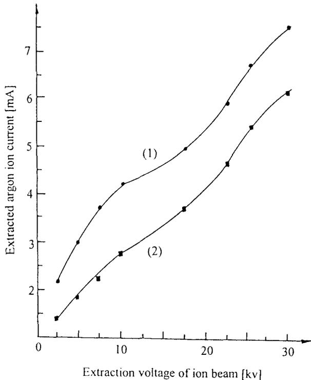
**Fig 6.** The extracted ion current as a function of extraction voltage.
