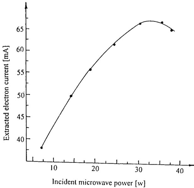
Fig 2. The extracted electron current as a function of the incident microwave power.
