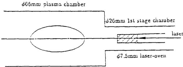
Fig.2 Schematic diagram of the laser oven in ECR2 ion source
