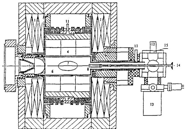
Fig.1 HIRFL 10GHz ECR2 ion source.
