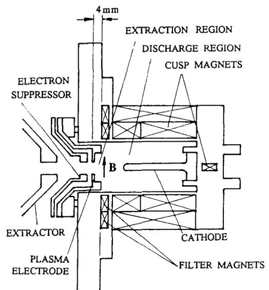
Fig. 1. Schematic view of the H<sup>-</sup> source.
