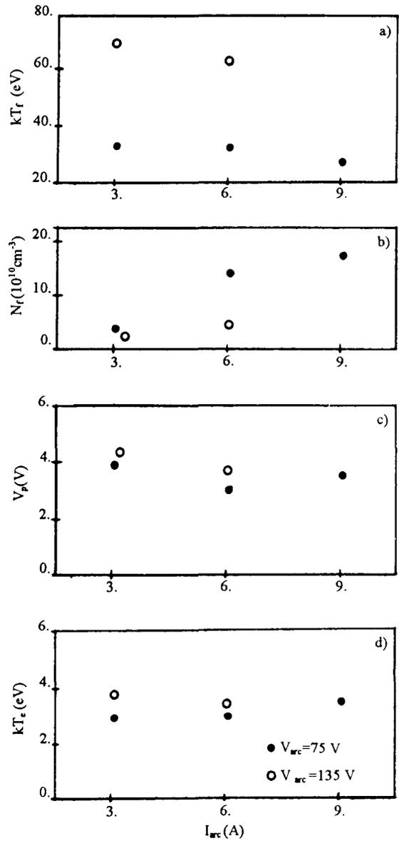
Fig. 4. Fast electron temperature - a) and density - b), plasma potential - c) and cold electron temperature - d) in the discharge region as functions of arc current.
