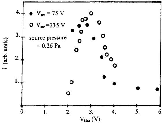
Fig. 2.  $H^+$  current as a function of plasma electrode bias.
