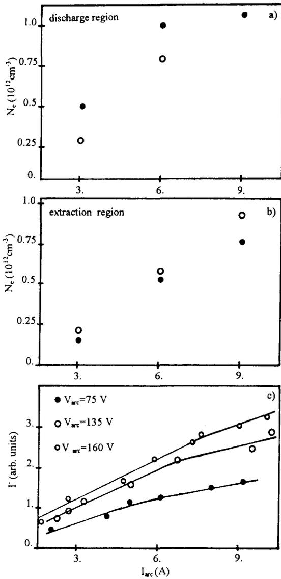
Fig. 3. Cold electron densities in the discharge region - a), in the extraction region - b) and  $H^+$  current - c) as functions of arc current.
