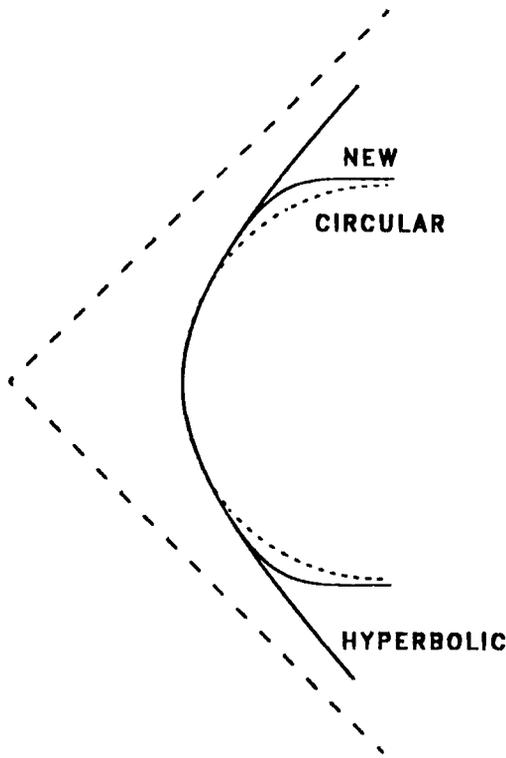
Fig. 2. Pole profile of a quadrupole obtained with the new method for  $C_{14}=0.00004$ . An optimized circular profile and an ideal hyperbolic profile are also shown.
