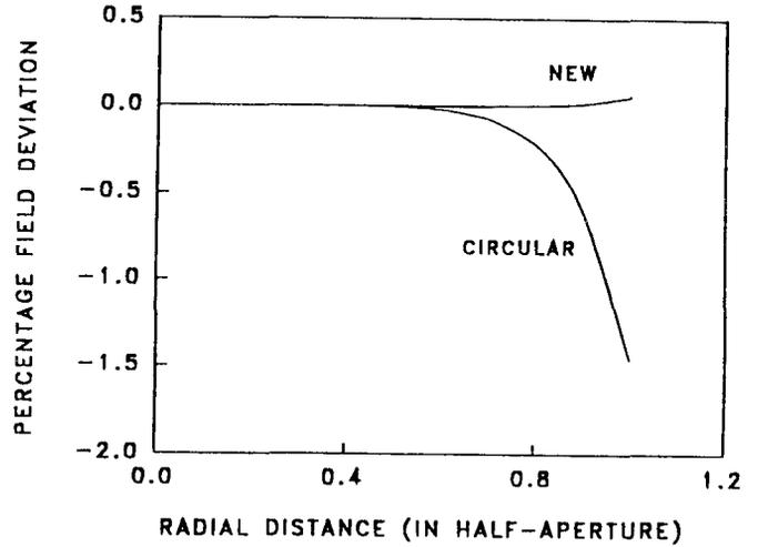
Fig. 4. Comparison of field error of the new profile with that of the circular profile
