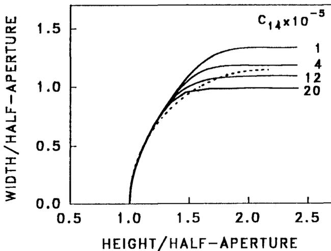
Fig. 3. Variation of the width of the new pole profile for various values of  $C_{14}$ .
