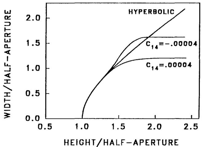
Fig. 5. Comparison of two pole shapes giving the same field deviation in amplitude but opposite in sign. The pole shape for positive  $C_{14}$  has a smaller pole width.
