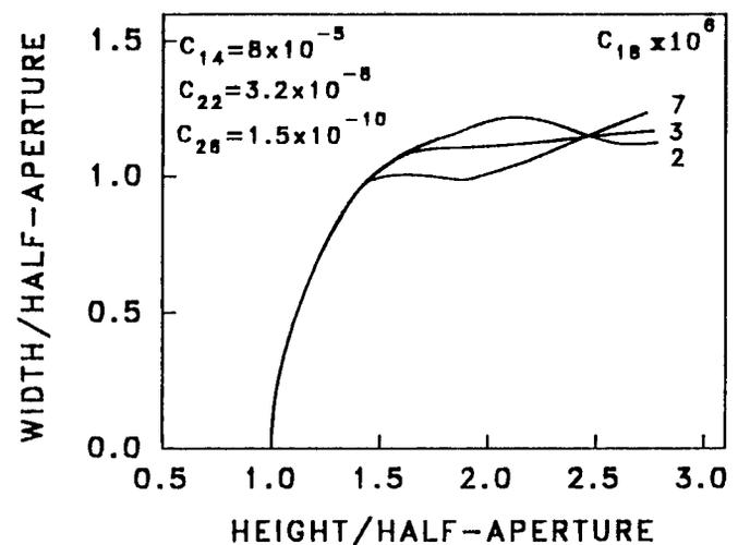
Fig.1. Change of pole profile as  $C_{18}$  changes
