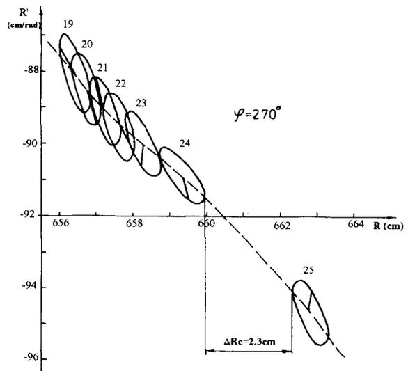
Figure 1: Results of the computer calculation beam particle extraction from the supercyclotron.
