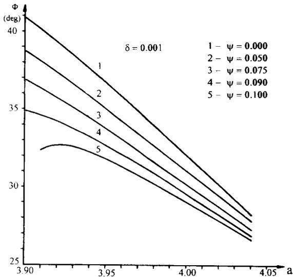
Figure 2:  $a = \frac{\Delta W_{01}}{\Delta W_{02}}$  - energy gain ratio,  $\Phi$  - beam phase width,  $\delta$  - relative energy spread,  $\psi$  - phase shift.
