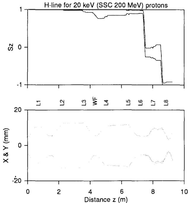
Figure 3: Calculation for polarized beam in the injection line. The beam emittance is 100 mm.mrad and the initial polarization is in the direction of the beam line. The upper plot shows envelopes of minimum and maximum spin projection along direction of travel, the difference between the two lines is the spread in polarization. The lower plot shows horizontal and vertical beam envelopes.
