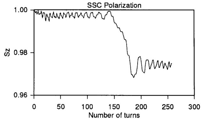
Figure 5: Calculation for 200 MeV protons in a field with mid-plane errors, obtained by displacing a sector magnet 1 mm vertically. The beam amplitude is 1 mm, and depolarization of a few percent is predicted at an energy near 114 MeV.
