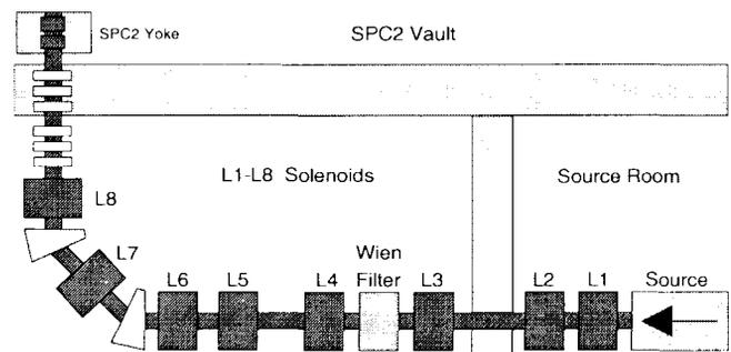
Figure 1: Schematic layout of the polarized beam injection line, showing the source and main beam line elements.
