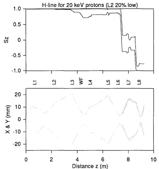
Figure 4: Calculation for the injection line with field setting of solenoid L2 20% too low. Polarization decreases to 75%.
