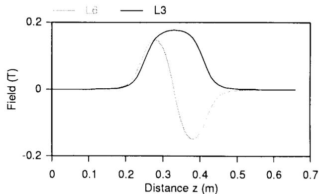
Figure 2: Fields measured along the axis, for two types of solenoids.
