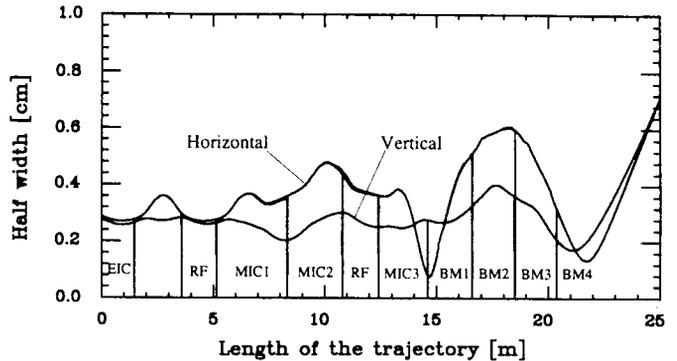
Figure 5: Envelopes of the injected beam, adjusted with gradient-field-coils.
