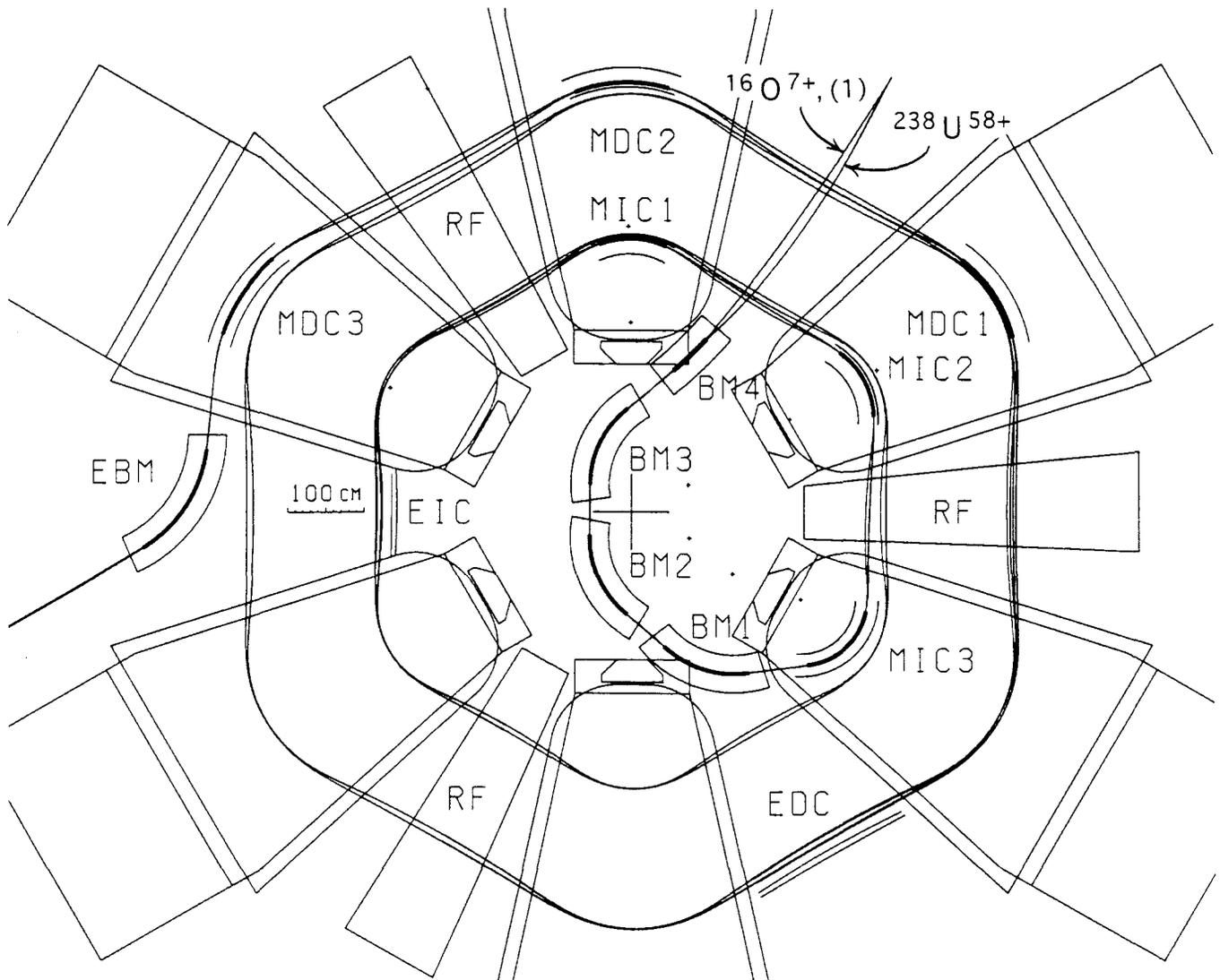
Figure 1: Schematic layouts of the injection and extraction elements and trajectories of two typical beams.
