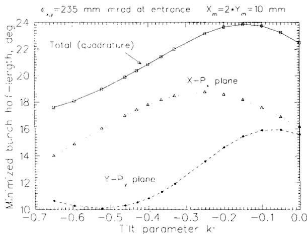
Figure 4: Minimized bunch length at the exits of inflexors providing the correct beam centering ( $x_m$ ,  $y_m$  fixed)
