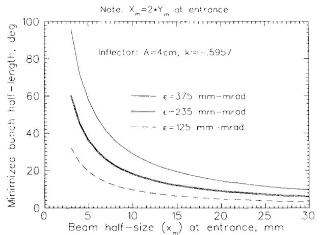
Figure 5: The effect of varying the beam size on bunch length for three different emittances
