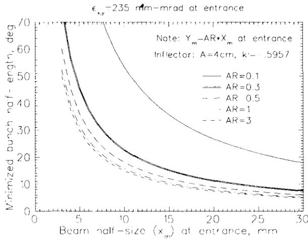
Figure 6: The minimized bunch length  $l(1)_{min}$  as a function of the beam aspect ratio at the inflector entrance
