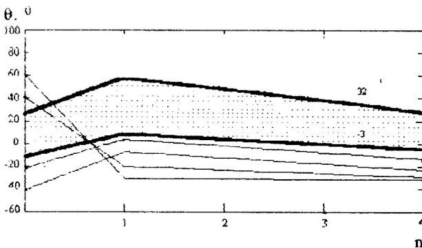
Fig.1. The dependence of initial ion phases  $\theta_0$  on the number of first half-turns n. Normal position of ion source,  $\alpha=0$ .
