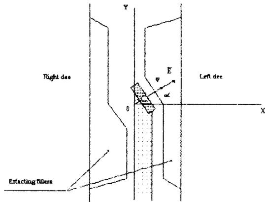
Fig.2. Ion source revolved on  $\alpha$  relatively extracting puller.
