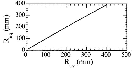
Figure 2: Correlation between the radial position of the equilibrium orbit in the direction of the main probe axis and the average radius for the 10 MeV proton beam.
