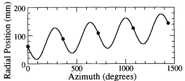
Figure 4: Radial positions(dots) from the first to the fifth turn of the 10 MeV proton beam. The curve accounts for the accelerated equilibrium orbit determined by the fitting.
