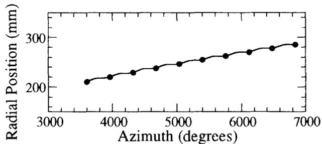
Figure 6: Radial positions(dots) from the eleventh to the twentieth turn of the 10 MeV proton beam.
