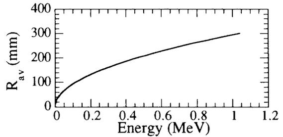
Figure 3: The average radius of the equilibrium orbit as a function of the particle energy for a 10 MeV proton beam.
