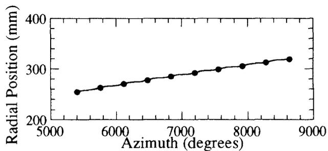
Figure 7: Radial positions(dots) from the sixteenth to the twenty-fifth turn of the 10 MeV proton beam.
