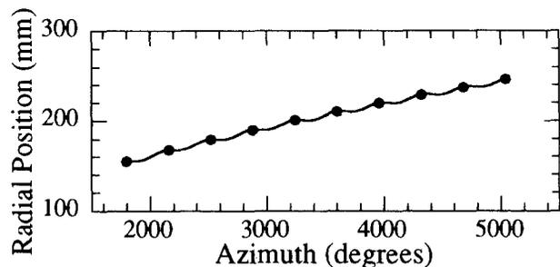
Figure 5: Radial positions(dots) from the sixth to the fifteenth turn of the 10 MeV proton beam.
