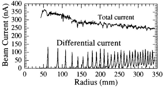
Figure 1: Beam density distribution for the 10 MeV proton beam measured with the main probe.
