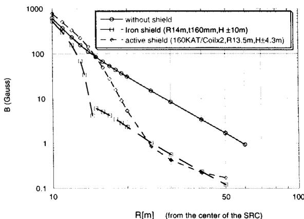
Figure 9: Leakage field distribution.
