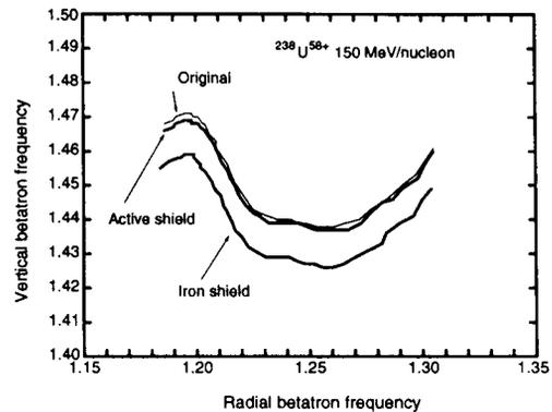
Figure 10: Effect of magnetic shield to betatron frequencies.
