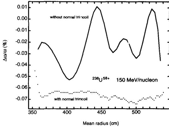
Figure 7: Effect of normal trim coil: frequency error to isochronous.
