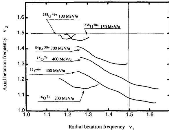
Figure 8: Working paths of typical ions.
