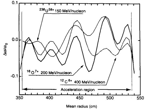
Figure 5: Frequency error to the isochronous condition.
