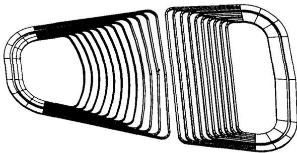
Figure 4: Configuration of the superconducting trim coils.
