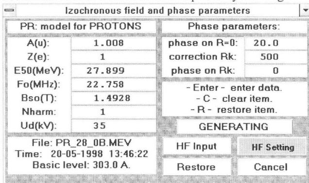
Figure 3. Window for the set-up of parameters of the accelerating regime.
