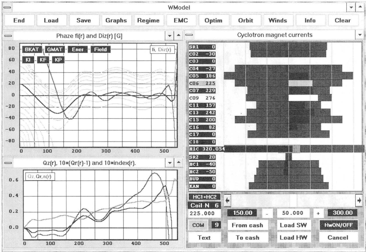
Figure 2. Main window for the cyclotron accelerating regime on-line control.
