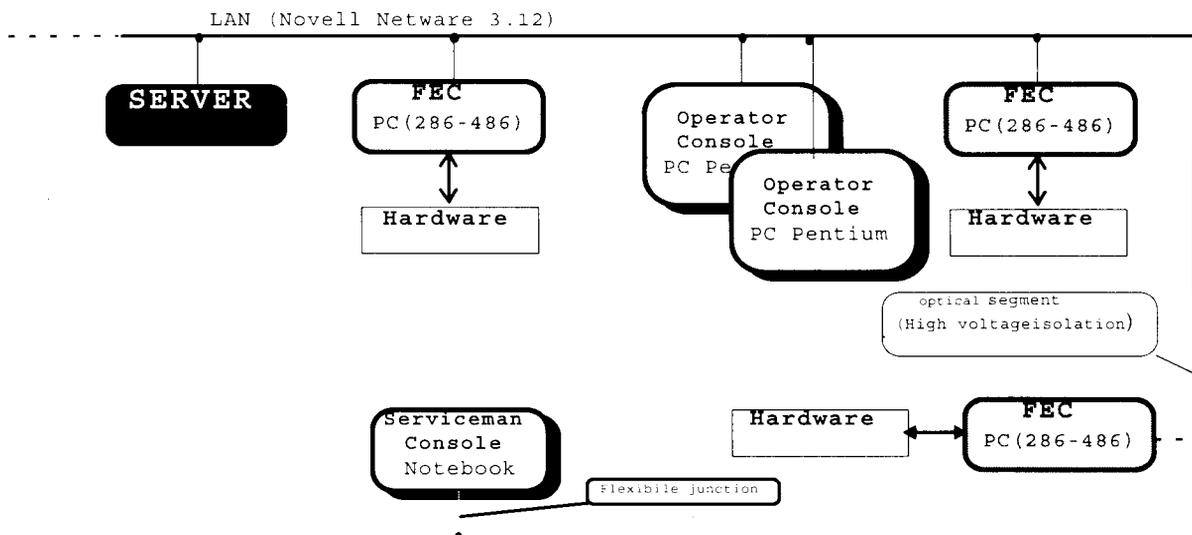
Figure 1. Structure of the ISOLDE-based control system
