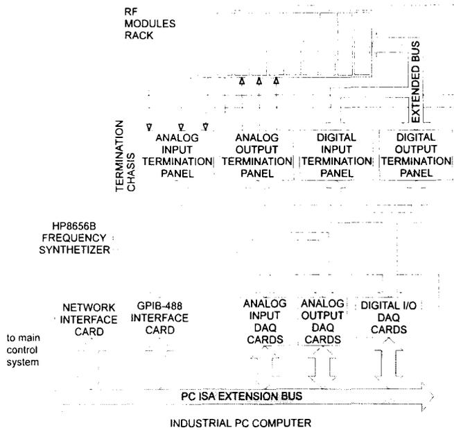
Figure 1: Interconnections between components of the RF control system and the industrial PC
