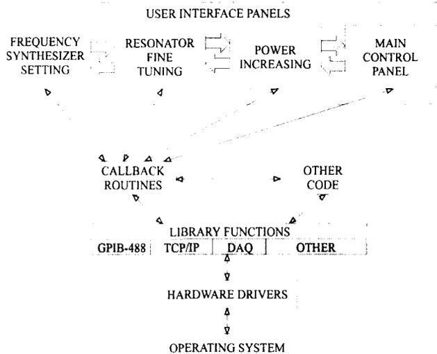
Figure 2: The RF Control System software architecture
