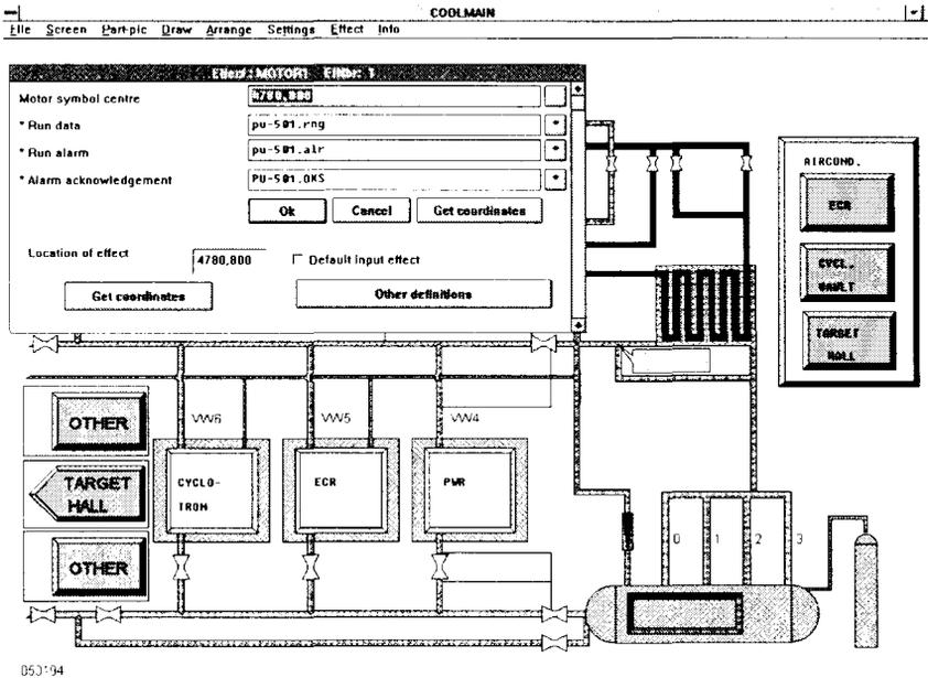
Figure 4: This figure shows how to define a pump effect in the graphics editor for the cooling system of the accelerator.
