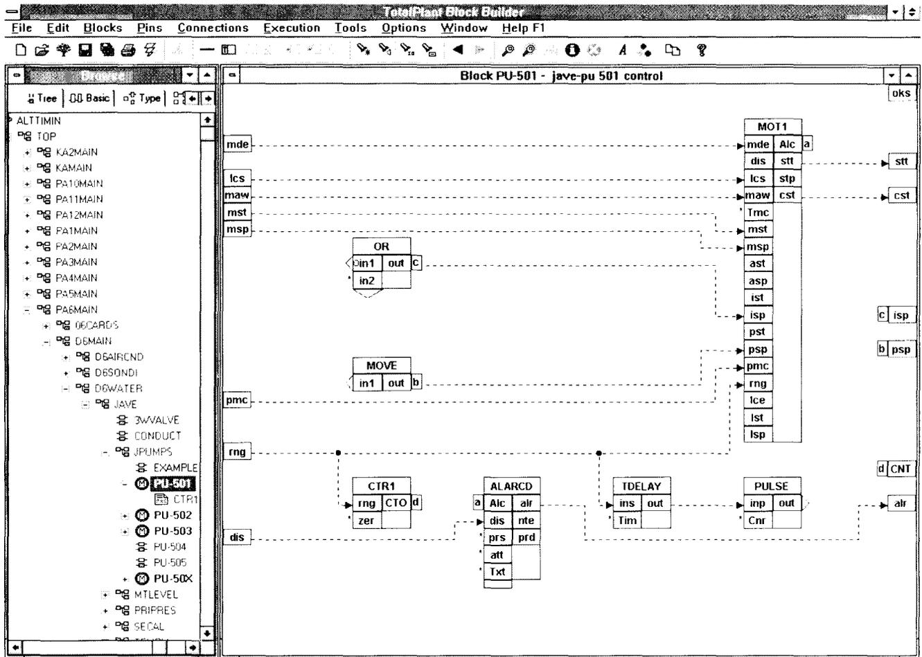
Figure 3: Cooling pump control program in the block editor
