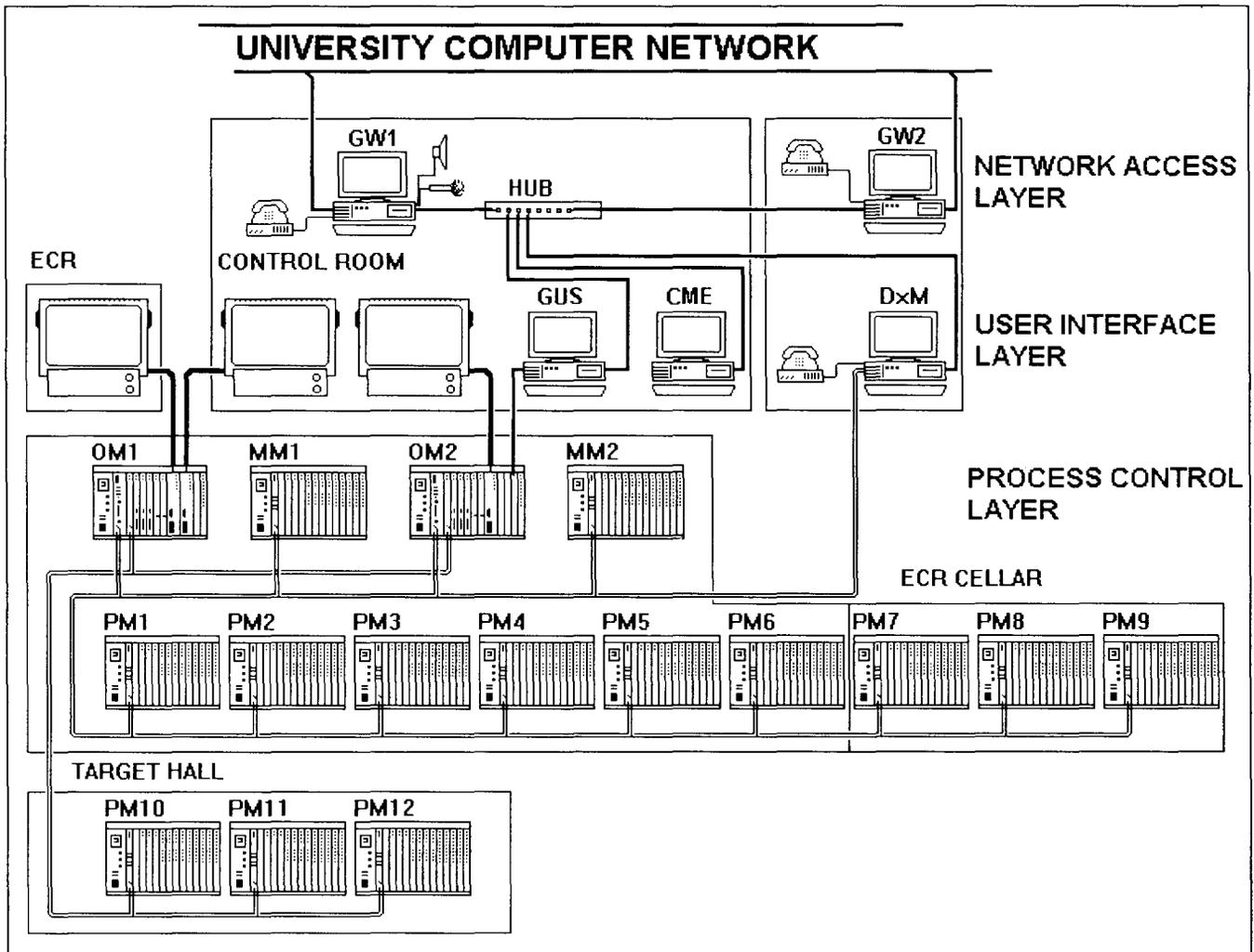
Figure 2: The hardware configuration of the control system in June 1998
