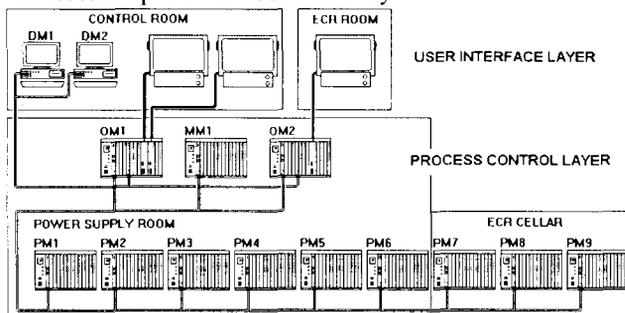
Figure 1: The hardware configuration in June 1990
