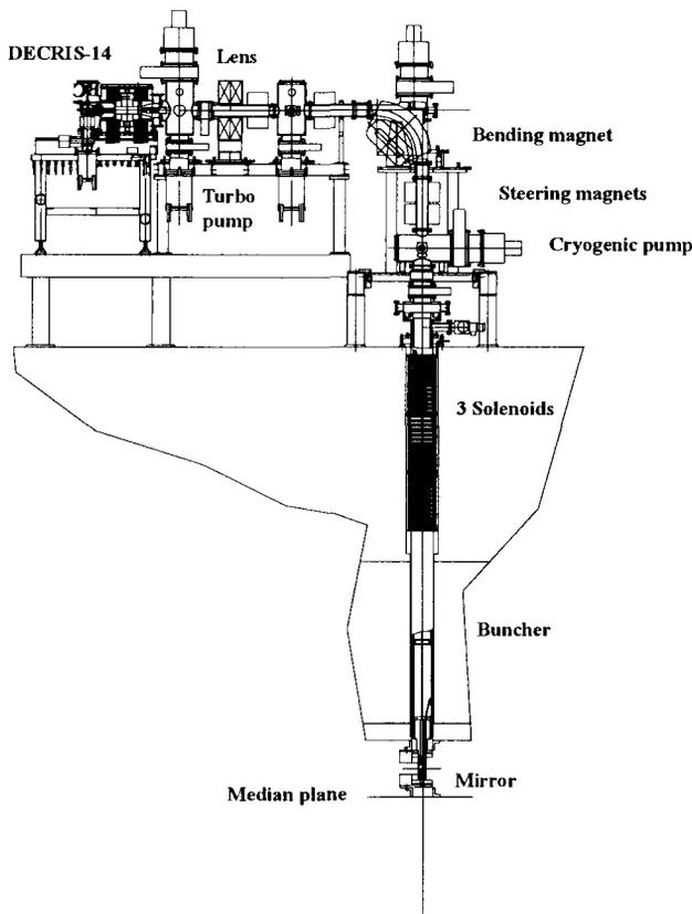
Fig. 4. The axial injection system of the U-400M cyclotron.
