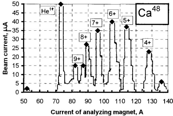
Fig.2. Spectrum of  $^{48}\text{Ca}$  from ECR4M optimized for  $^{48}\text{Ca}^{5+}$ .
