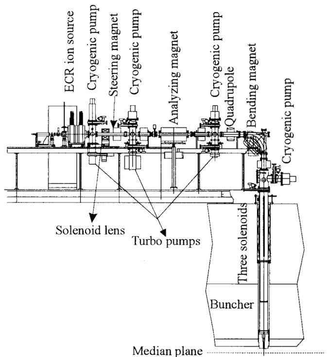
Fig. 1. The axial injection system of the U-400 cyclotron
