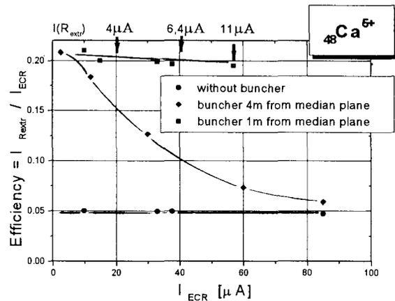
Fig.3. Efficiency of phase capture and acceleration in the cyclotron U-400 without buncher and with buncher installed in 1.1m and 4m from the median plane. ( $I_{R_{extr}}$  - accelerated beam current at the final radius,  $I_{ECR}$  - injected beam current)
