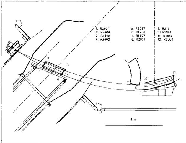
Fig. 6. Lay-out of the components of the beam extraction system and the beam trajectory.
