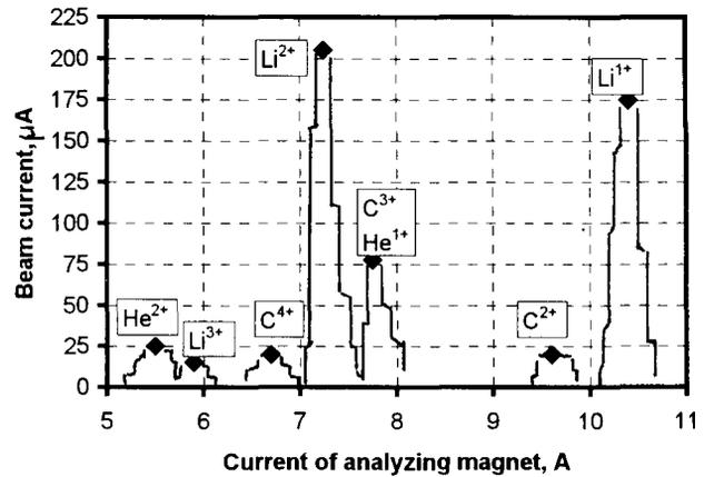
Figure 7. Li spectrum optimized on the maximum current of  $\text{Li}^{2+}$  beam required for acceleration.
