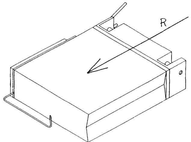
Figure 3: perspective view of radial probe head with measuring wire
