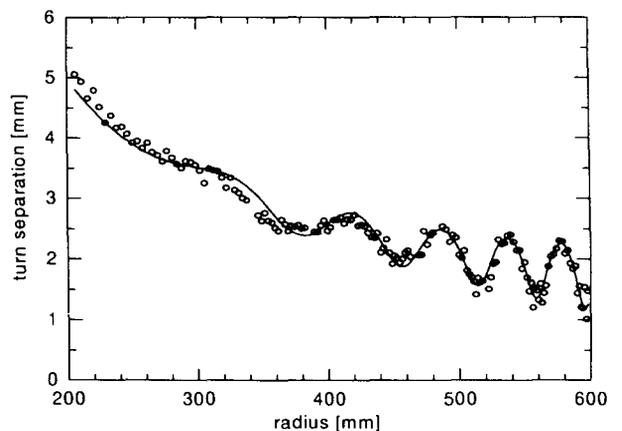
Figure 7: radius gain per turn as a function of radius scan displaying separated turns to R=600mm, a plot, shown in figure 9, was made of the radius gain per turn as a function of radius. The modulation is caused by a coherent radial oscillation. Using  $v_r$  values, obtained from field maps, the radial gain per turn can be calculated. The
