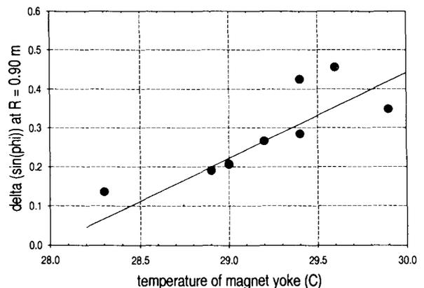
Figure 9: field corrections as a function of yoke temperature
