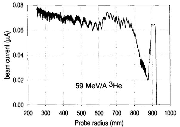
Figure 6: radial probe (block) current vs. radius for 59 MeV/A  $^3\text{He}$  beam
