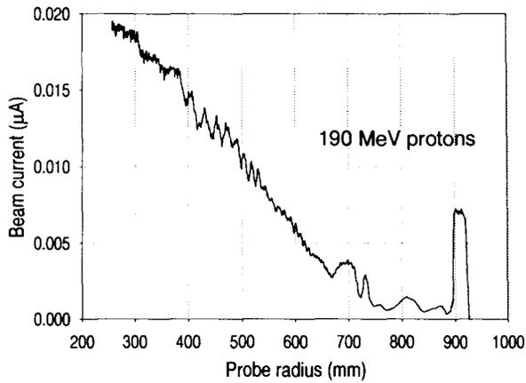
Figure 4: radial probe scan for 190 MeV protons: current on block electrode
