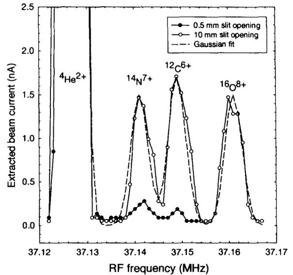
Figure 8: beam current as a function of rf-frequency; ion-source gas:  $\text{CO}_2$  and He
