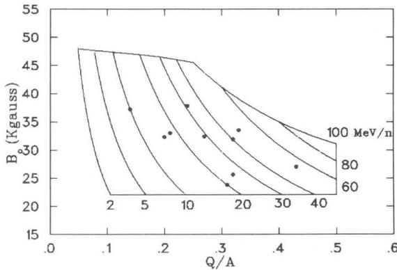
Figure 1: Operating diagram of the Superconducting Cyclotron: distribution of the beam types developed to date
