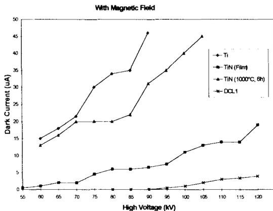
Figure 4: Electrostatic properties of different electrodes of the deflectors
