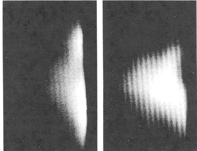
Figure 2: Off-centered (left side) and centered (right side) beam at the extraction radius ( $R_{\text{probe}}=870$  mm)
