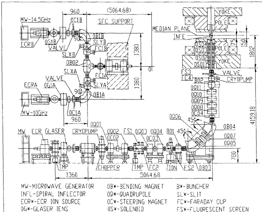
Figure 3, New axial injection beam line for SFC
