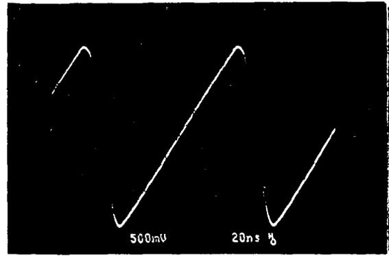
Figure 4, Sawtooth waveform of B02 ( $f=6\text{MHz}$ )
