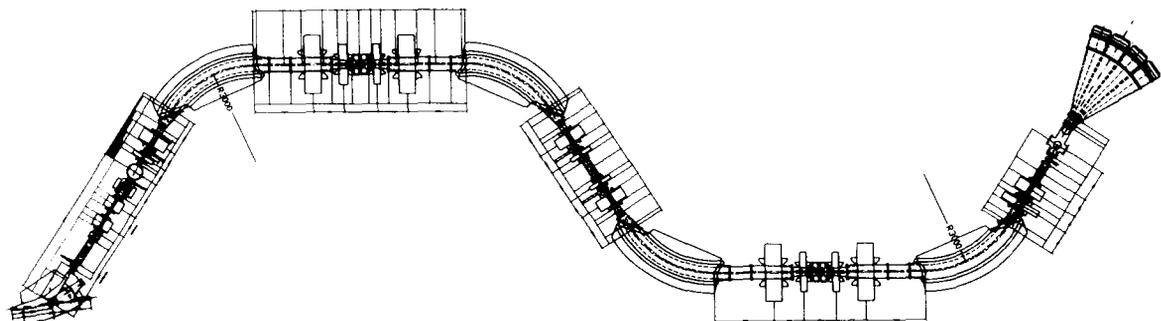
Figure 2, Layout of radioactive ion beam line RIBLL
