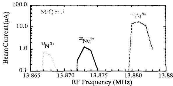
Fig. 5 :Dependence of the beam intensity on the RF frequency for the M/Q=5 cocktail beam. The absolute values of the beam current depend on the tune of the ECR ion source.
