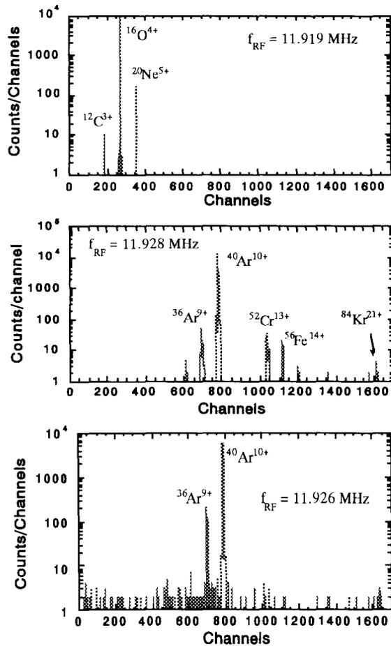
Fig. 6 : Pulse height spectra of the M/Q=4 cocktail ions measured with a SSD. The spectra were obtained at three RF frequencies.
