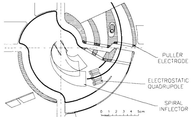
Figure 2: The position of the electrostatic quadrupole in relation to the spiral inflector and the puller electrode of SPC2.
