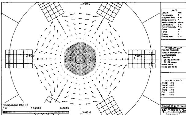
Figure 3: The ionisation region which has been computed for the magnet configuration of an ECR-ioniser designed for our polarized ion source, employing stronger and twice as thick permanent magnets for the hexapole field than those at PSI [6].
