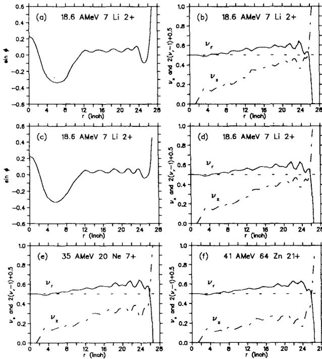
Fig. 3. Graphs of  $\sin\phi$  and  $v_r$  and  $v_z$  versus radius for: (a)-(b) 18.6 AMeV  ${}^7\text{Li}^{2+}$  (an earlier solution), (c)-(d) 18.6 AMeV  ${}^7\text{Li}^{2+}$ , (e) 35 AMeV  ${}^{20}\text{Ne}^{7+}$ , and (f) 41 AMeV  ${}^{64}\text{Zn}^{21+}$  beam. Beams are extracted at about 26.5 inches.
