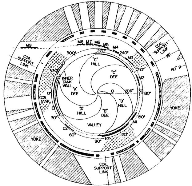
Fig. 2. Median plane of the K500 cyclotron.
