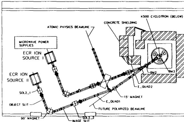
Fig. 1. Two ECR ion sources and the injection line above the cyclotron.
