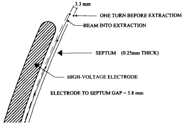
Fig. 4. Beam at extraction showing the turn separation and the trajectory into the deflector. The dashed line represents the midline through the electrode to septum gap.
