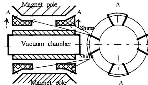
Fig. 1: The installation of steel shims.
