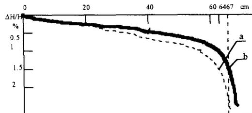
Fig. 2: The radial distribution of the average magnetic field (a – without shims, b – with shims).
