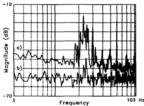
Figure 2: FFT spectrum of the beam position signal at injection. a) loop "off"; b) loop "on".
