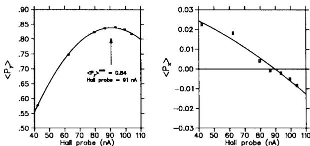
Figure 4: Wien Filter Tuning. At a magnetic field corresponding to a Hall probe reading of 40 uA, transverse polarization of the injected beam is about 60%, and of extracted beam 2.5%.
