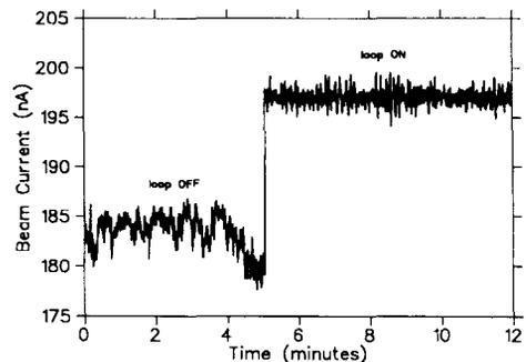
Figure 3: Current stabilization system operation.
