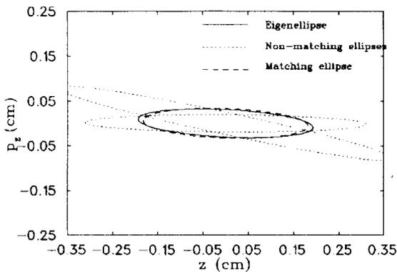
Figure 7: Matching in the vertical plane from the inflector exit towards extraction
