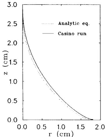
Figure 2: Central ray trajectories inside the inflector: vertical motion
