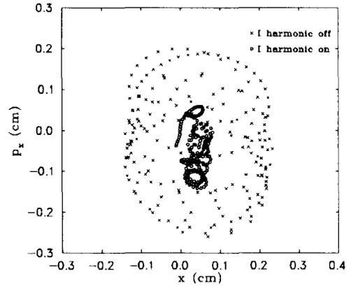
Figure 5: Off-centering correction by means of a 1 harmonic bump
