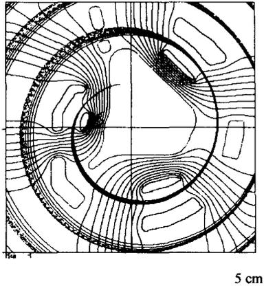
Figure 3: The 2<sup>nd</sup> harmonic central region of the LNS Superconducting Cyclotron. Central trajectories with starting times from 200° to 235° are plotted.
