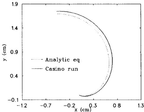
Figure 1: Central ray trajectories inside the inflector: projections on the median plane.
