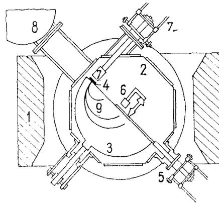
Fig.1. Test band. 1-magnet, 2-vacuum chamber, 3-Dee, 4-puller, 5-moving probe, 6-Faraday cap, 7-source, 8-vacuum pump, 9-ion orbits.
