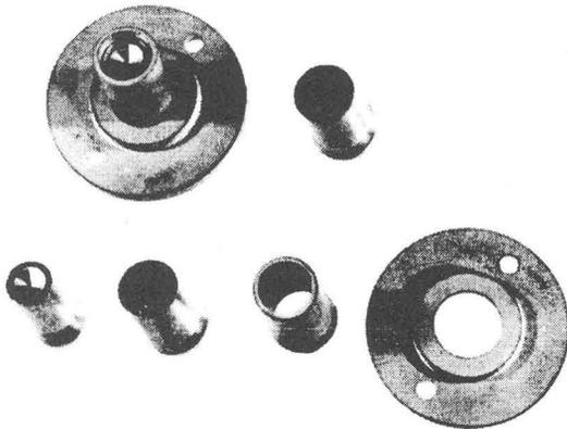
Fig.2. Cathode and anticathode assembly
