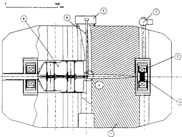
Figure 3 : Cross section of the cyclotron through a hill and a RF valley
