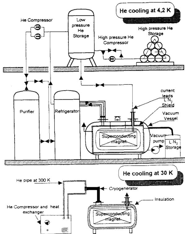
Figure 1 : Cooling circuit
