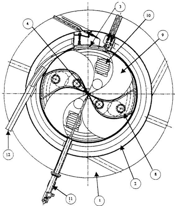
Figure 2 : View of the cyclotron in the median plan
