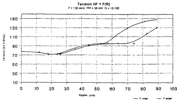
Figure 4: RF voltage distribution
