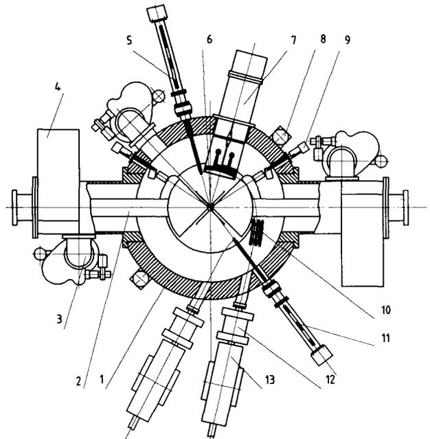
Fig.3. The lay-out diagram of the new cyclotron design. 1. Electromagnet. 2. Resonance system. 3. Diffusion aggregate. 4. HF final stage. 5. Beam probe. 6. Ion source. 7. Deflector. 8. Lift. 9. Trimmer. 10. Magnetic channel. 11. Stripping device. 12. Positioning magnet. 13. Lens.
