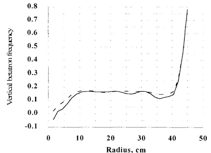
Fig. 2. Frequency of vertical oscillations in the mode of protons' acceleration up to energy of 22.5 MeV. Dashed line is the same for 20 MeV energy
