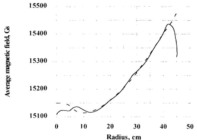
Fig. 1. The curve of shaped magnetic field of 450 A coil current. Dashed curve shows isochronous field for an energy of 22.5 MEV
