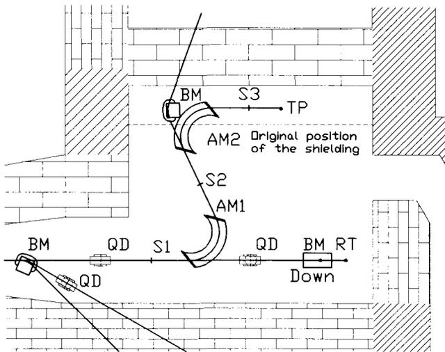
Fig.2. The tandem of  $115^\circ$  analysers in the beam transport system
