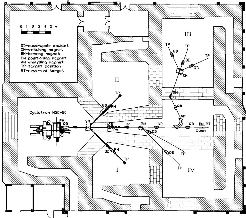
Fig.1. Layout the first (bold) and second stages of the beam transport system
